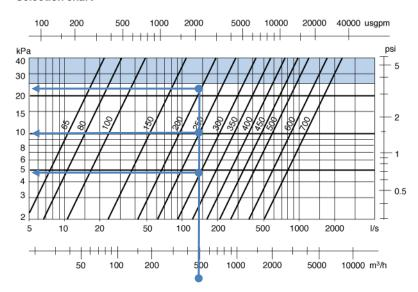
The relation between flow rate and pressure drop over the Bernoulli Filter is shown in the selection chart above.
