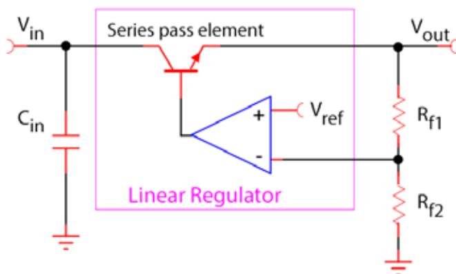
Figure 1. The linear power supply uses an all-analog closed-loop feedback approach to control the pass element, such that the supply output voltage tracks the internal reference voltage. In the block diagram, the voltage divider at the right-hand side allows the user to set the output-voltage versus reference-voltage comparison ratio.
