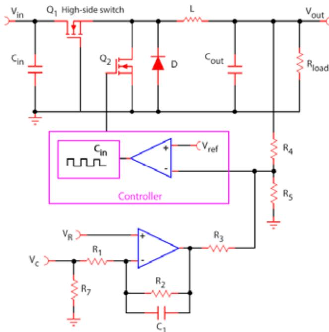
Figure 2. In the SMPS supply, the output voltage is regulated by clocked on/off pulse-width modulation of the pass element, resulting in low losses and high efficiency, but the output has clock noise that must be filtered to establish a clean DC output voltage.
